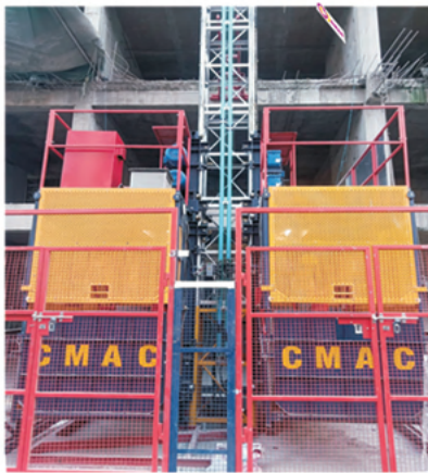
PM Hoist Double Cage, Hyderabad
